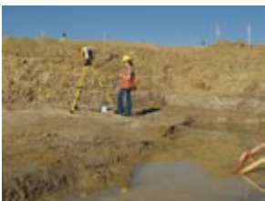
Trimble GX enables real-time progress monitoring on a construction site with volume and surface computations. For large sites, OverScan™ technology provides greater range.
