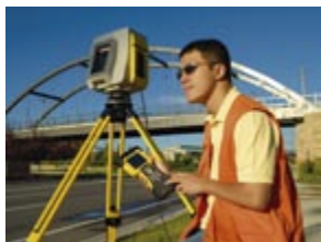
On traditional survey jobs the Trimble GX provides enriched data for future reference and faster deliverables. Additionally, DR technology reduces safety hazards for you and the public; capture dense data at a safe distance from the scene; this is ideal for civil infrastructure...and no lane closures required.
